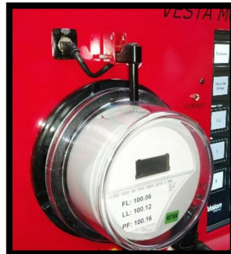
*Itron Centron™ meters can be tested without the use of a movable arm. The sensor is aligned when the meter is mounted in the socket.*
