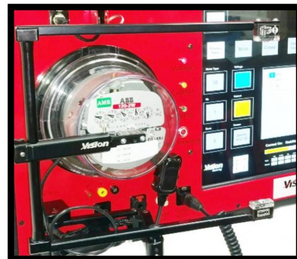
*While Vesta comes with an adjustable arm, it should only be necessary for testing mechanical meters either through the holes in the disk or on the disk edge.*
