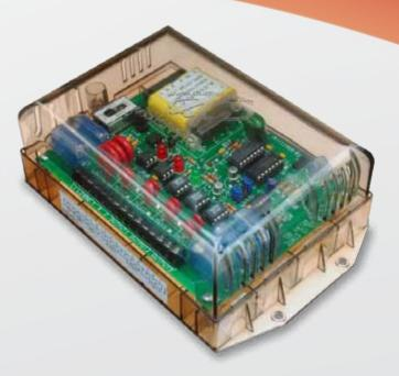
The Sentry 50 Isolation Relay provides an electronically isolated interface between the ouput of the utility meter and the electronic measuring equipment such as Data Recorders, Totalizers and Demand Monitoring Equipment. It accepts either a 2-wire Form A or 3-wire Form C open collector or relay contact input and provides three Form A or Form C isolated outputs.
